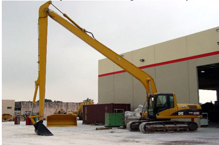
Figure 4. Typical long reach excavator with 60-foot boom.
