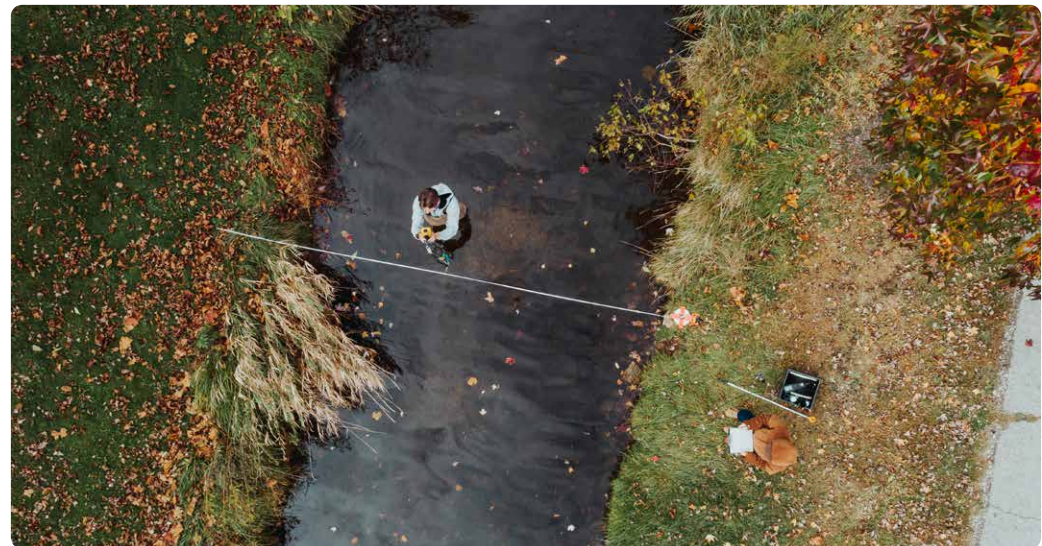
Clockwise from top left: A stream sensor box houses electronics and a solar panel to ensure consistent data collection. College interns record data. Flow, depth, oxygen, and other parameters are collected across the entire width of a stream..
