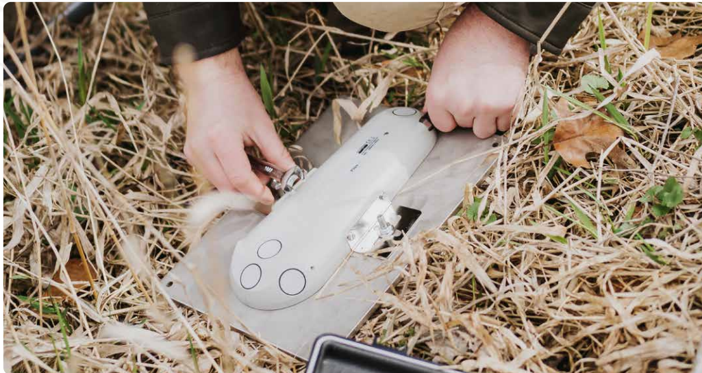
Above: Normally, this part of the stream sensors is hidden below the surface of a stream. It captures data at regular intervals and sends it back to the computer above ground, and then sent to our website.
